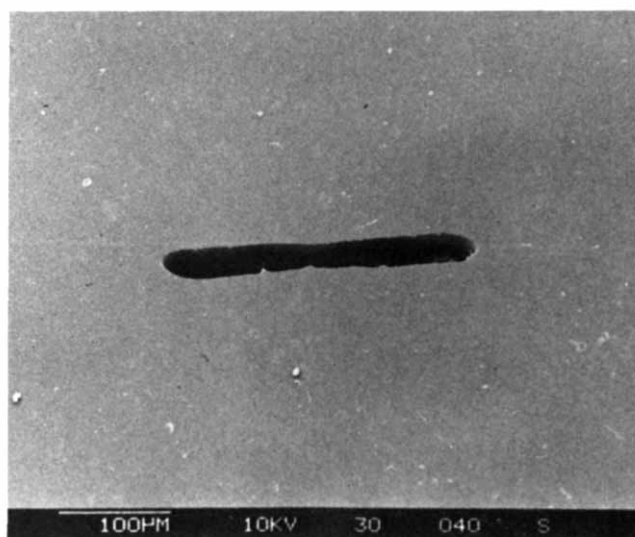
Fig. 6. Unbonded region in the polished section after partial sintering (sample 6 joined with ethyl acetate).
